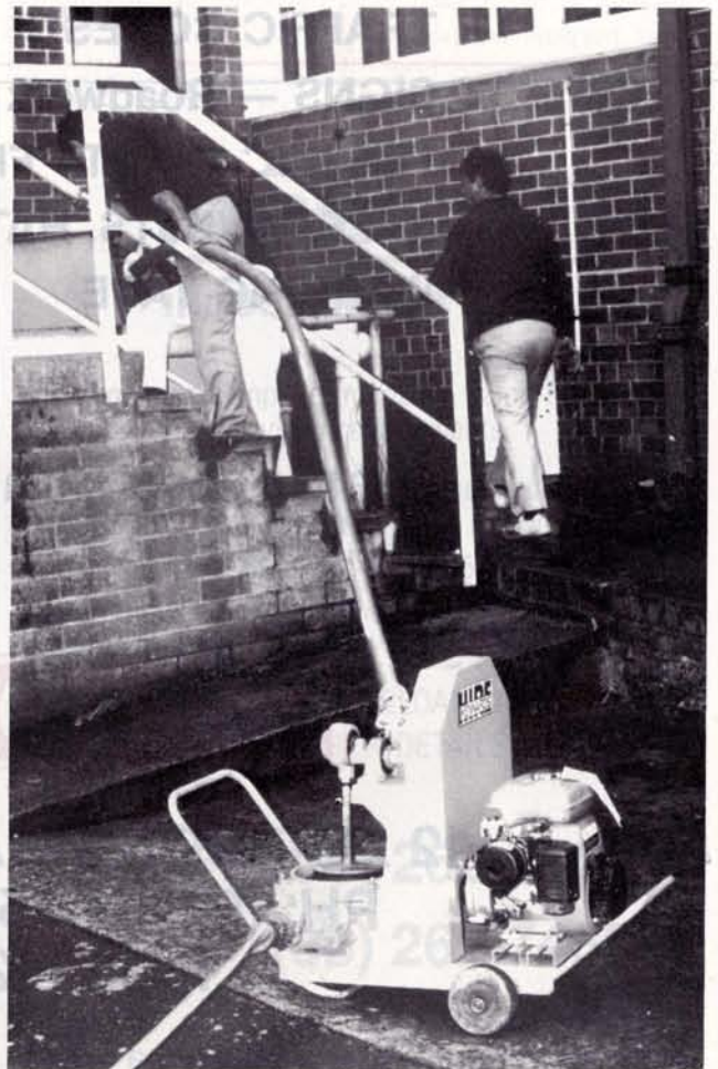
A diaphragm pump from Kennards Hire empties a settlement tank at a major Sydney Hospital.
